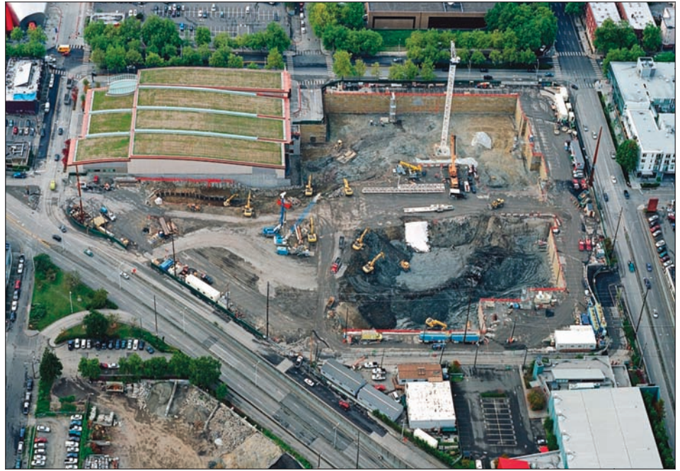
The Gates roof has five inches of soil over a layer of synthetic drainage.
